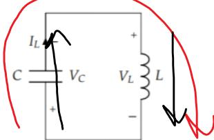
This is sometimes called an *LC* tank and we will derive its response in this problem. Assume at  $t = 0$  we have  $V_C(0) = V_s = 1$  V and  $\frac{dV_C}{dt}(t = 0) = 0$ . Also suppose  $L = 9\text{nH}$  and  $C = 1\text{nF}$ .
