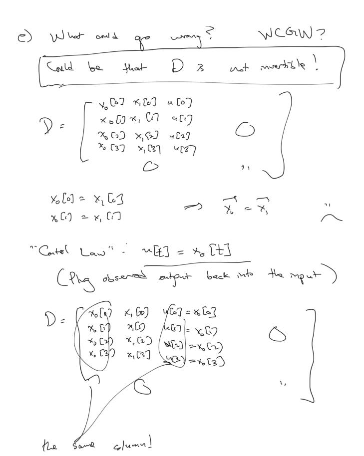
By poor choice of inputs, we messed up the Sustem ID ( have to be careful)
