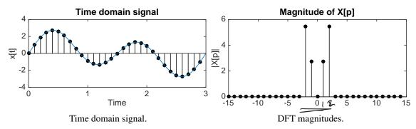
Now, we have obtained the DFT coefficients for another sampled signal, with sampling frequency of 6Hz:
