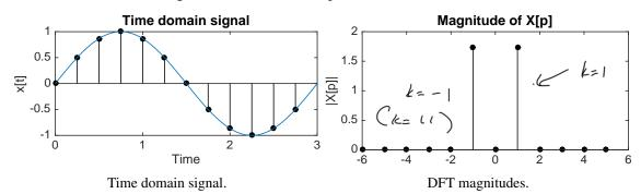
Now, we have sampled the same signal at a different sampling rate to get 30 samples over 3 seconds:
