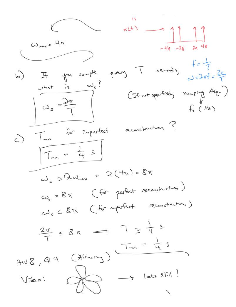
30 fps ( sampling at 30 fps ) a) fan is still, what could freal be? · 1 of a rotation looks the same as O rotating 2 of a staton E rotation would look the same f = 30 Hz  $T_S = \frac{1}{f_S} = \frac{1}{30}$ Fred = K/S rotations = K/S Ts seconds = 1/30 s = 6k Hz 5) 3 blads fapparet 2 2 HZ freq = fapparent + (contribution from "looks still")  $= 2Hz + \frac{413}{T_s}$ | free = 2+10k Hz |
