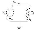
Let  $V_s = 5$  V and  $R_1 = 1 \Omega$ . Use nodal analysis to solve for the power dissipated or supplied by each element.
