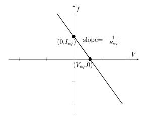
Notice that the V-intercept is given by  $(V_{eq}, 0)$ . What circuit element has 0 current flowing through it? An open circuit!
