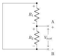
We hook up a voltage source  $V_{test}$  across the terminals A and B. We could measure out  $I_{test}$ , but in this case, we can already see the equivalent resistance without any more math!
