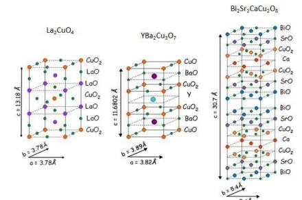
oxide sandwiched between ions (like lanthanum, barium, strontium). These ions dope electrons into the copper oxide layer and become Mott insulators themselves.
