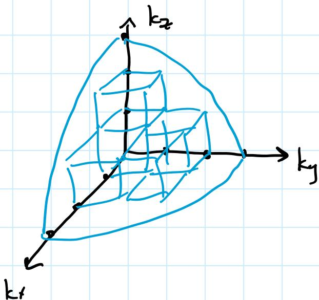
The electrons fill up k-space, starting from the center and settling into the next - lowest energy state (combination of  $k_x, k_y, k_z$  that's not already taken and has the next lowest energy).
